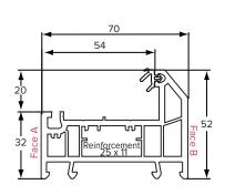
546816 586816 (Foiled white base) 586815 (Foiled coloured base) **CHAMFERED SLIM OUTER** FRAME 52MM (5 CHAMBER)
