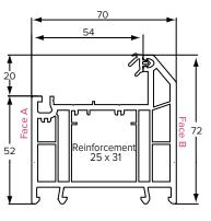
546836 586836 (Foiled white base) 586835 (Foiled coloured base) CHAMFERED LARGE OUTER FRAME 72MM (5 CHAMBER)
